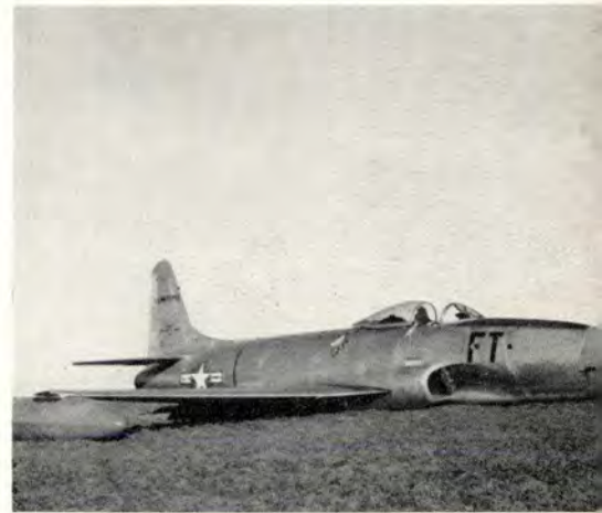
Modern high stress cockpit design and use of shoulder harness and protective helmets enable pilots to walk away from wheels-up landings. The pilots of these three fighters chose favorable fields for emergency landings
